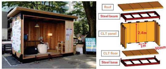
Figure 6: Photo of the CLT module (left); schematic diagram of the module's structural system (right).
