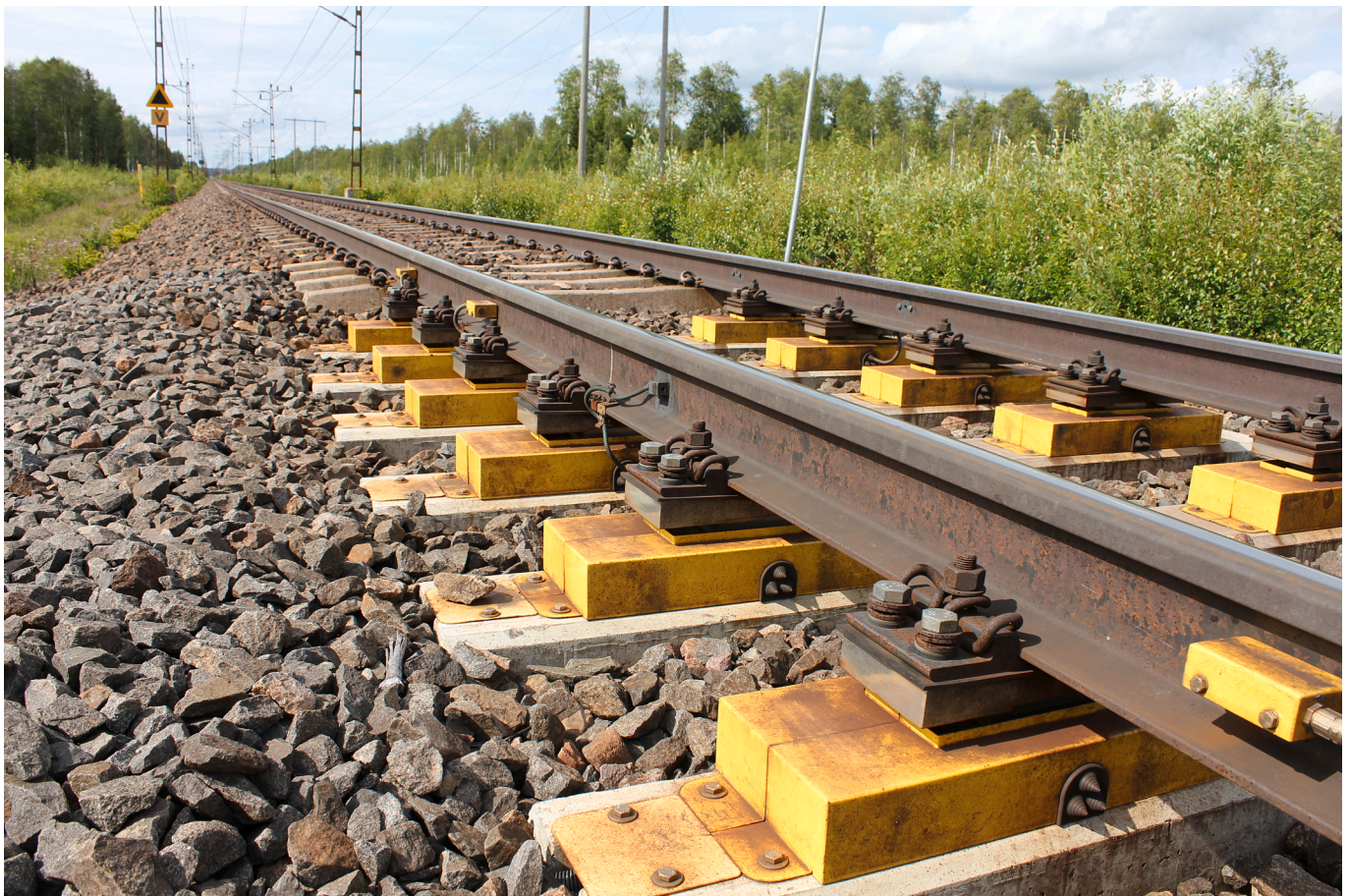
Fig. 3. Wheel impact load detector at Sunderbyn on Malmbanan [15]. Rail seat loads are measured at eight consecutive sleepers. Photo by Matthias Asplund, Swedish Transport Administration.
