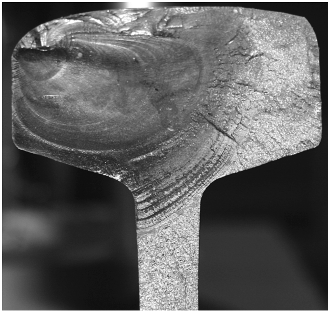
Fig. 1. Head check crack (initiation top left) propagating to transverse growth and causing a rail break (light grey area indicating final fracture).
