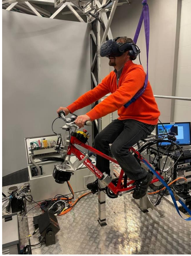
Figure 4- Bike simulator with virtual reality headset
