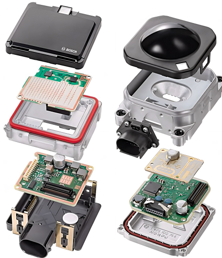
Figure 3.3: Exploded view of the Bosch RADAR sensors [71].
