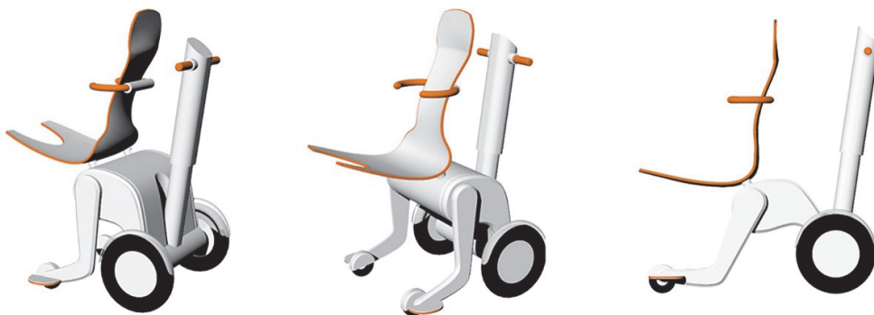
Image 2. Initial AT concept, i.e., model A with an integrated socket in the seat.
