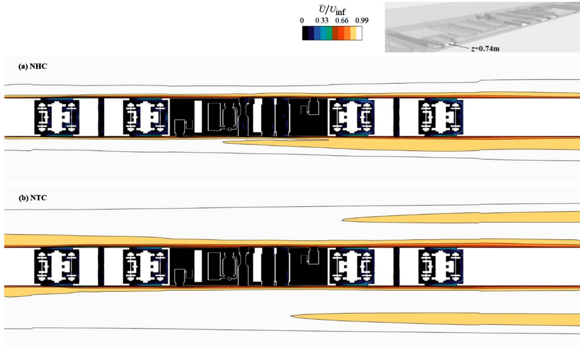
Figure 14. The time-averaged velocity contour of the EC in the z = 0.74 m plane in (a) near head car and (b) near tail car conditions.
