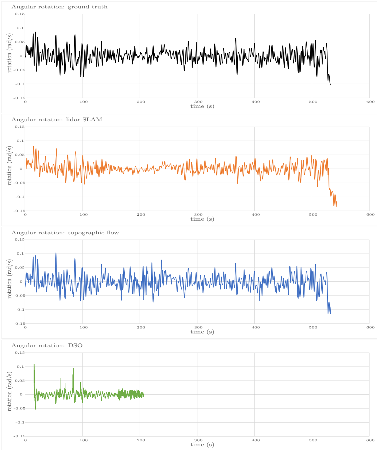
Figure 5.6: The angular velocity ( \text{rad s}^{-1} ) of the ground truth, lidar SLAM, topographic flow, and DSO algorithms. Note that in the case of the DSO, no more data was available after 210s, due to a logging error.
