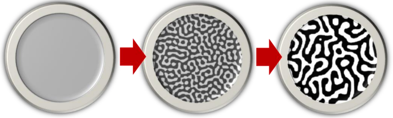
Figure 6. Schematic illustration of the progress of spinodal transformation over time.
