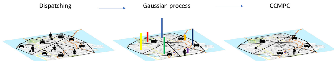
Fig. 3. Visual representation of the dispatching, travel demand prediction, and MPC. The map is split into N stations and there is an initial number of requests and vehicles. First, the requests are matched with vehicles in the same station. Then the travel demand is predicted, here represented by the colored bars. Based on the travel demand prediction the AMoD optimization problem is solved (Algorithm 1) and the vehicles are rebalanced accordingly.
