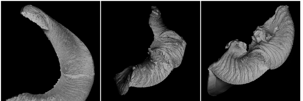
Figure 5.2: Chips from Face Turning 1 (left), 2 (middle), 3 (right).
