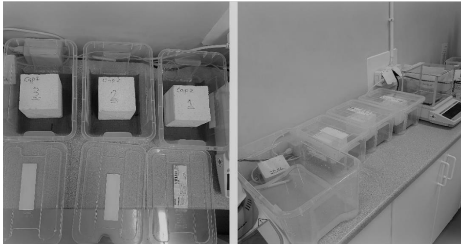
Figure 3. The experimental set up where each sample, placed in separate and closed container, was in contact with water with a minimum water level of 5-10 mm. The water mass gain was weighted manually by a scale for 90 minutes.
