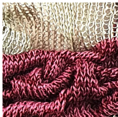
Figure 2-13. Hanging stitches technique. Left: an illustration of the principle of the knit. Right: a section of a prototype knitted with the technique, using wool (pink) and linen (beige) yarns
