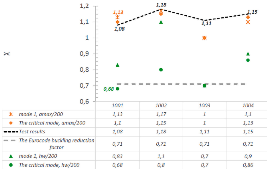
Fig. 17. Shear buckling factors obtained from imperfection sensitivity studies in comparison to the conducted tests and the Eurocode design model.
