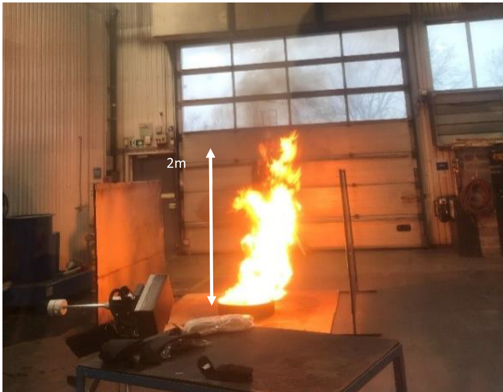
Figure 3. Photo of the experiment. The lidar device located in the lower left portion of the photo is aimed at the flame. The laser beam passes through the flame, giving rise to strong elastic light scattering, and is then terminated on a screen located behind the flame.
