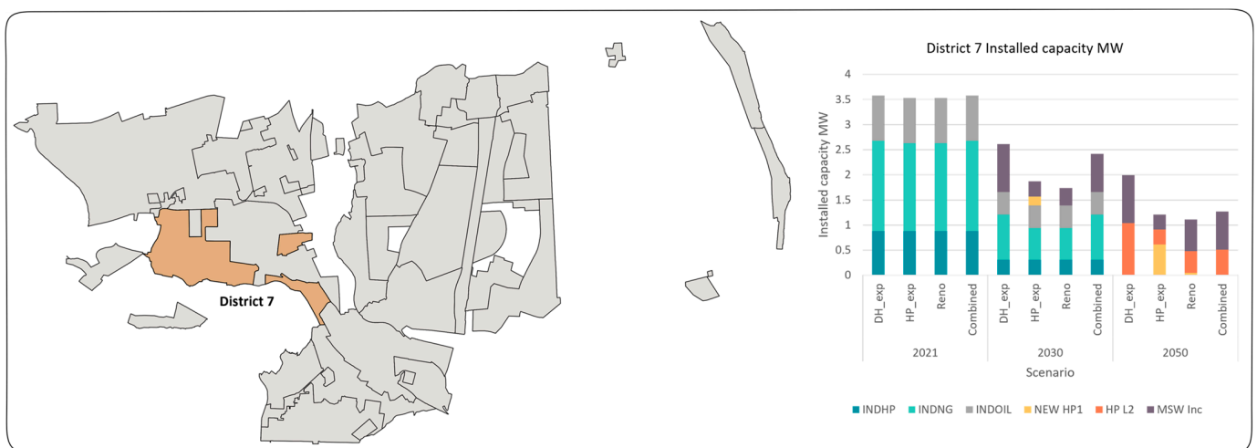
Figure 10. The evolution of the installed heating technology capacity in District 7 for the four scenarios. DH_exp, DH expansion scenario; HP_exp, HP subsidy scenario; Reno, renovation scenario; Combined, combined scenario.
