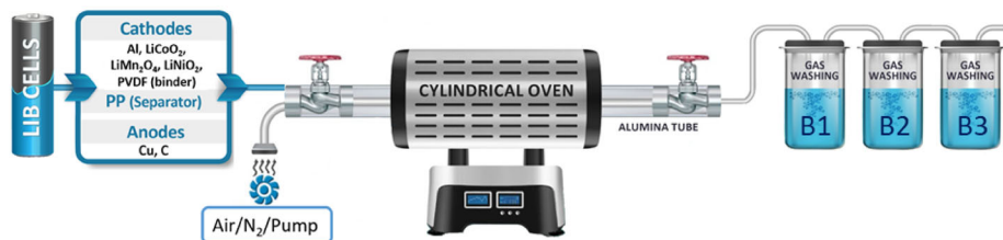
Figure 1. Apparatus with the washing system used for the simulation of the thermal accident.
