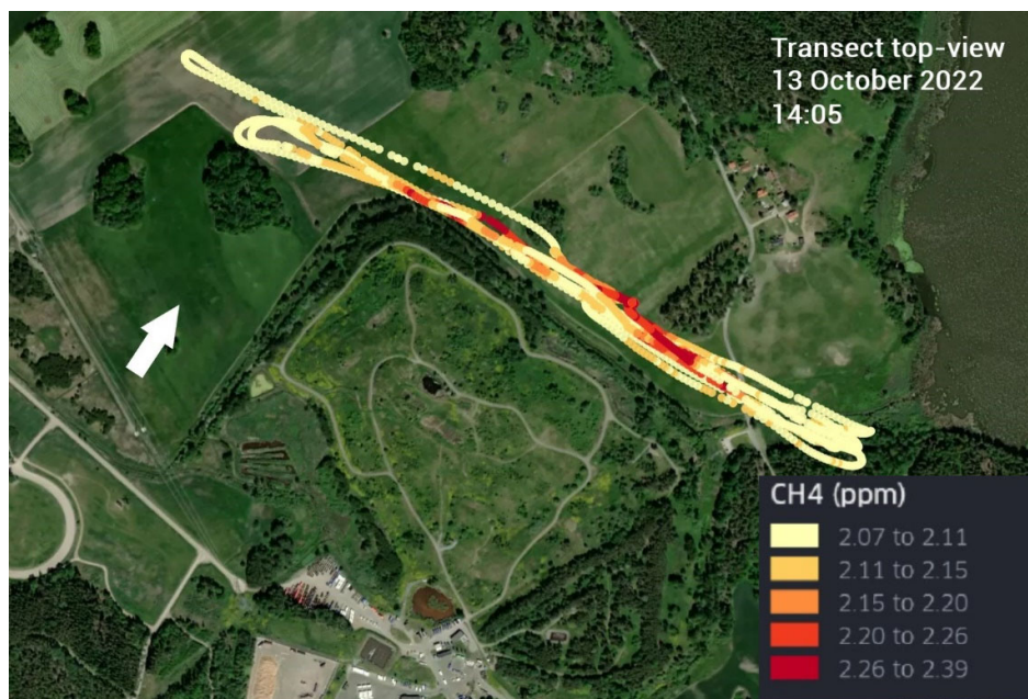
Figure 6. Visualization of the performed measurement transects while carrying out drone-based laser measurements using the wall approach at Landfill A1 on October 12, 14:05. Graphic from: www.kepler.gl © with underlying Map from Mapbox©.
