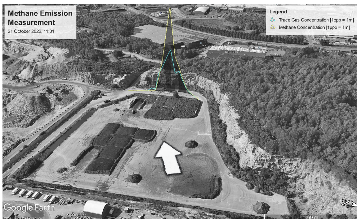
Figure 21. Example of a drone-based laser sensors measurements of methane and tracer concentrations at the external sludge storage location on October 21, 2022, carried out at 12:10. See Figure 3 for a general description of the graph structure. Map: Google Earth™ © 2022.
