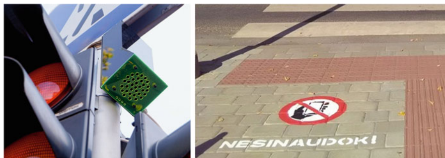
Fig. 7 Audible and visual means to draw the attention of pedestrians using phones at pedestrian crossings
