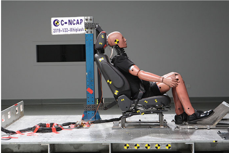
Fig. 8 Typical whiplash seat sled test setup with the BioRID-II dummy, used by many NCAPs around the world including IIHS, Euro NCAP, JNCAP, and China NCAP
