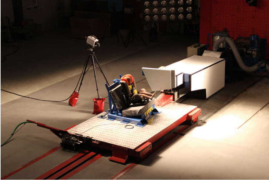
Fig. 7 Side impact test setup used a.o. by the European Testing Consortium to evaluate the protection offered by Child Restraint Systems
