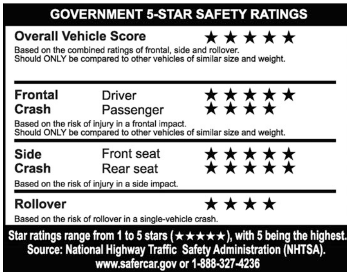
Fig. 2 US NCAP safety rating information published by NHTSA is required to be part of the Monroney (automobile price sticker) label
