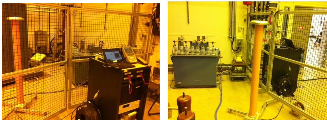
Figure 3-25. IGBT full bridge converter, step-up high voltage transformer and high voltage wide band voltage divider
