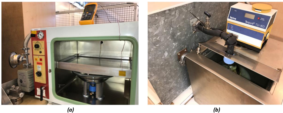
Figure 3-9. Dry oil preparation setup: A heating and vacuum chamber equipped inside with a steel tray for drying and collecting the dried oil (a), and the regulated hot water bath feeding the hot oil through a needle valve into a heating and vacuum chamber (b)
