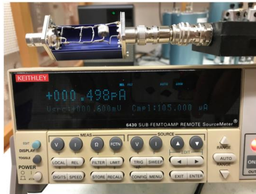
Figure 3-6. Test setup for verification of overvoltage protection system
