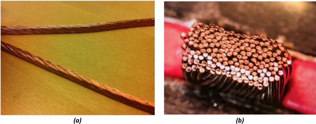
Figure 2-32. A rectangular litz wire and its strands: A rectangular litz wire (a), and a bunch of enamelled strands (b)
