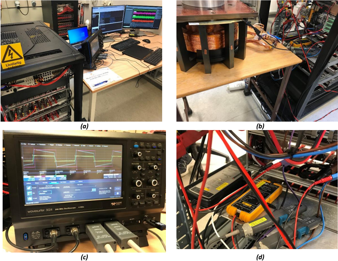
Figure 5-15. The DAB setup for recording the wave of the prototype MF: the DAB and control and recording setup (a), the MFT under test(b), the four-channel oscilloscope for recording the wave form (c) and the voltage and current probes for accurate acquisition of the waveforms (d)
