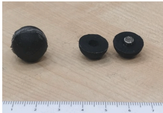
Fig. 2. A. Particle size distribution of the bed material used in the experiments, i.e., glass beads with a mean particle size of 106 \mu\text{m} and density of 2,486 \text{kg}/\text{m}^3 . b. Image of tracer particles, showing the cavity that holds the permanent magnet.
