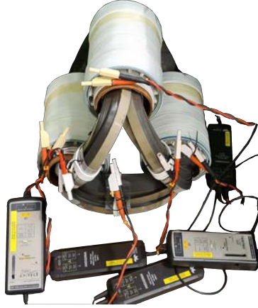
Figure 8.7: The experimental setup for measuring flux waveforms.
