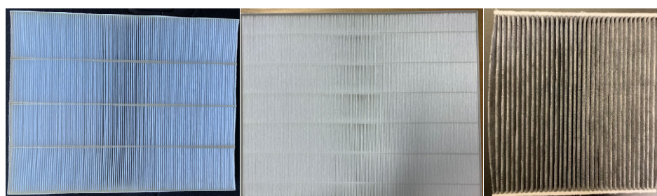
Figure 5 Prototype filters. Left: P1, Middle: P2. Right: original HVAC filter
