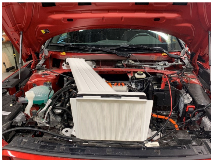
Figure 6 Filter prototype installation in an existing production vehicle's thermal bay
