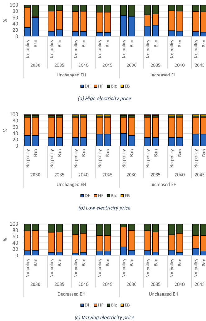
Fig. 4. The figure presents the modeling results as shares of heat energy supplied by the different technologies for new large single-family housing for the LEB heat load profiles in the cases of a climate policy not being implemented (No policy) or a ban on the use of fossil fuels (Ban) in the indicated years. EH, Excess heat; DH, district heating; HP, heat pump; Bio, biomass boiler; EB, electric boiler; LEB, Low-energy building.
