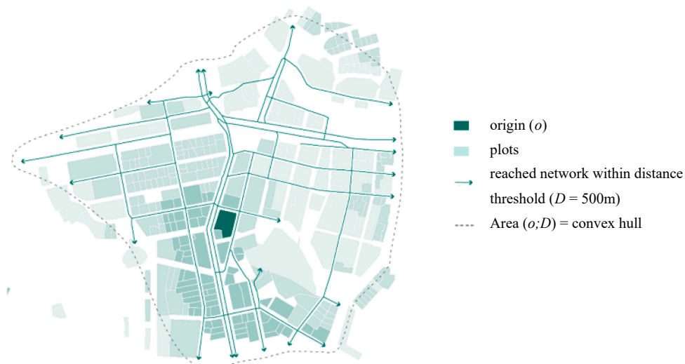
Figure A1. Definition of the convex hull used in PST for calculating Area(o; D) .
