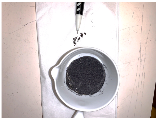
Fig. 6. Partial agglomeration of the braunite oxygen carrier.
