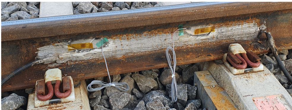
Figure 30. A full Wheatstone bridge mounted on the neutral axis of the rail web
