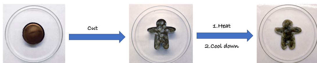
Fig. 7. (a) Optical microscopy images showing the process of self-healing on GSDZ5 hydrogel samples. (b) Photos showing that the GSDZ hydrogels can be remolded. R.T. stands for room temperature.
