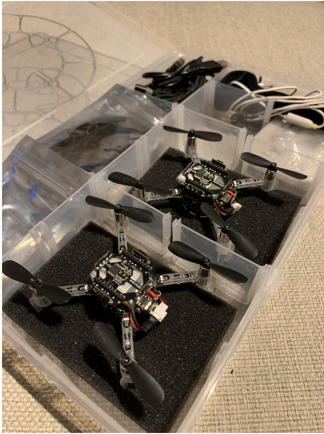
Figure 9: A photograph of the first prototype box showing two Crazyflie drones, a Bitolino respiration sensor, other accessories, and spare parts.
