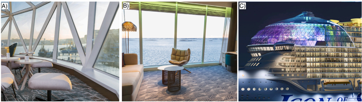
Fig. 1. Examples of insulating glass units in cruise ships. (A) and (B) are from Mein Schiff 2, and (C) is the Aqua Dome of Icon of the Seas. Source: Courtesy of Meyer Turku Oy.
