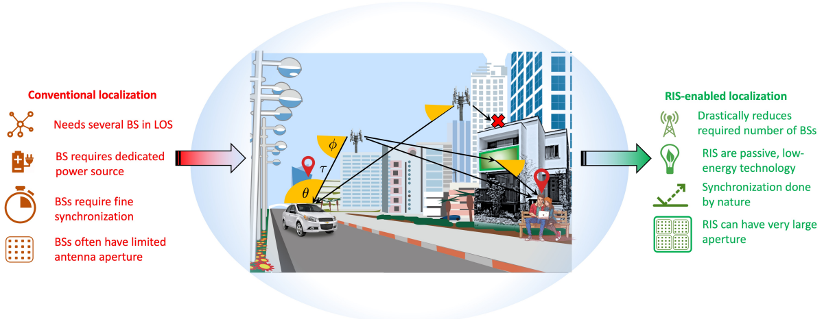
Fig. 1: RIS-enabled localization: without RIS, several BSs are needed for localization, while with RIS, localization is possible with less infrastructure. The symbols \tau , \phi , \theta are used to indicate ToAs, AoDs, and AoAs, respectively.
