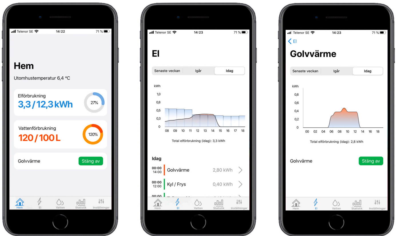
Fig. 1. Ero 2.0 in light mode. Home screen showing momentary electricity consumption and daily water use with possibility to control floor heating (left), electricity screen showing total consumption for appliances connected to smart plugs and floor heating in relation to the personal electricity threshold (middle) and electricity screen with appliance specific consumption (right).
