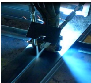
Figure 8: Roller with silica based woven textile Refrasil® wool. From Holder (2011).
