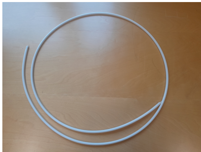
Figure 2.5: A 1 meter foam-cladded PMF with a solid rectangular cross-section (1.2 mm by 2.1 mm).
