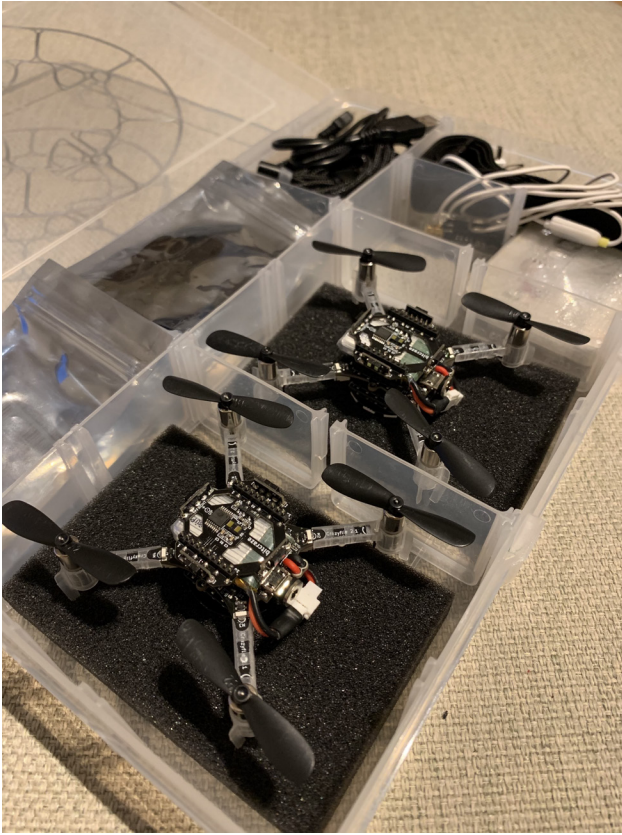
Figure 9: A photograph of the first prototype box showing two Crazyflie drones, a Bitalino respiration sensor, other accessories, and spare parts.
