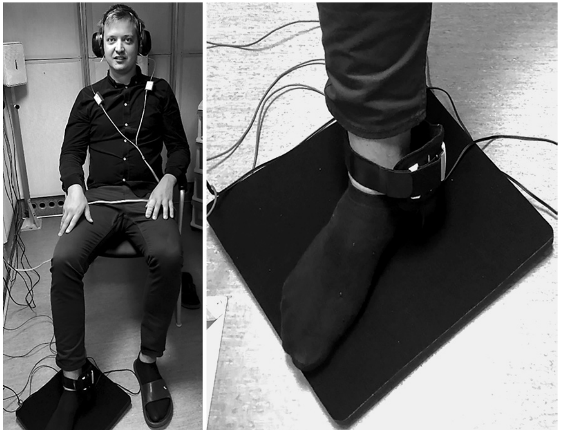
Fig. 1. Test setting for AA. The B250 was placed in contact with the medial malleolus with a velcro band, with an adjusted tension corresponding to a pressure at contact point of 10 N. The subjects during testing wore hearing protection against air conducted hearing contamination and disposable foam ear tips in connection with audiometer to deliver masking noise to the not stimulated side ear.
