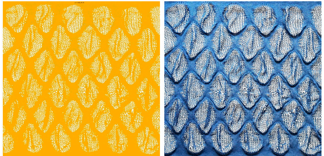
Figure 6. Porosity calculated by using a script in Processing (based on pixel darkness). The calculated porosity is illustrated through coloring pixels that count as solid, here represented in yellow.
