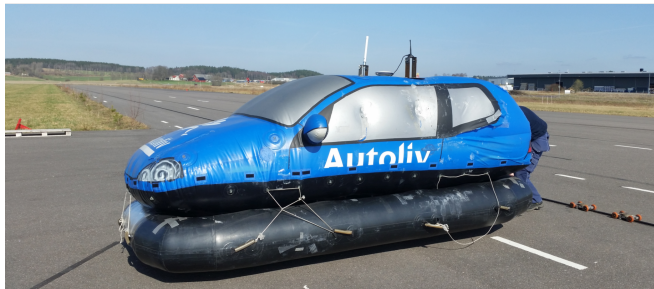
Figure 2.4: Test-track data collection on an airfield in Vårgårda, Sweden (a), using a robot cyclist (b) and a robot oncoming vehicle (c). Figures adapted from Rasch et al. (2020a) and Rasch and Dozza (2022).
