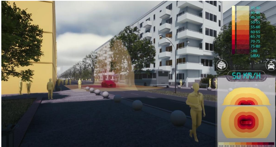
Figure 2: Illustration of the visualisation/auralisation tool in use with dynamic real-time noise levels illustrated with transparent coloured surfaces.
