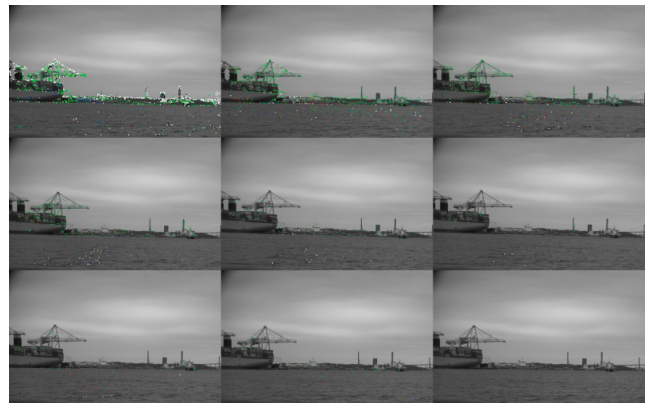
Fig. 3. A maximum of nine keyframes were used in the DSO algorithm and they are shown in the figure. The oldest keyframe is presented in the upper left corner and the most recent in the lower right corner. A large number of feature points are being tracked, managed, and labelled as candidate , active , and finally, marginalised when lost. In the figure, it can be seen that the crane provides a considerable amount of possible visual tracking features.
