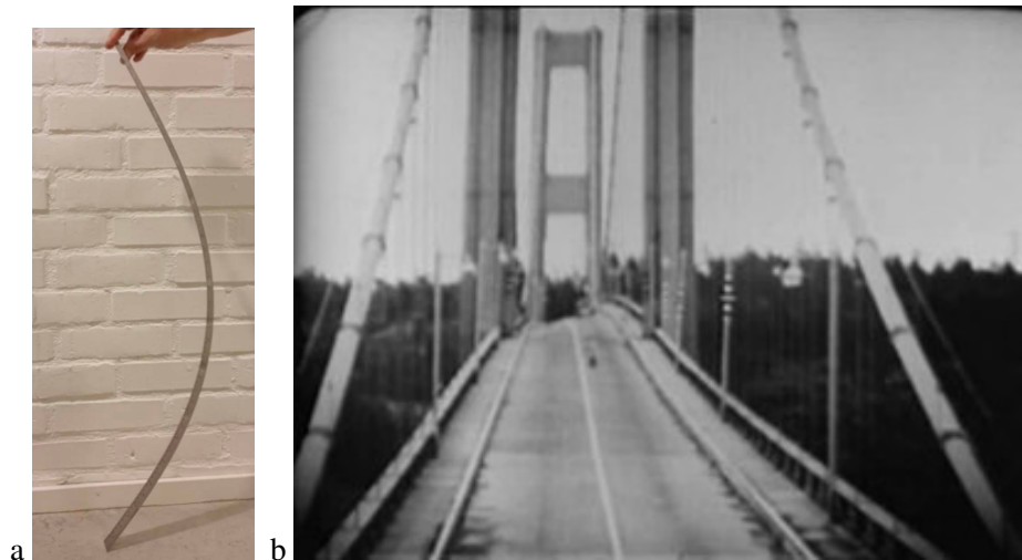
Figure 2: a) Euler buckling (Euler-2) and b) Dynamic instability (Tacoma Narrows bridge).
