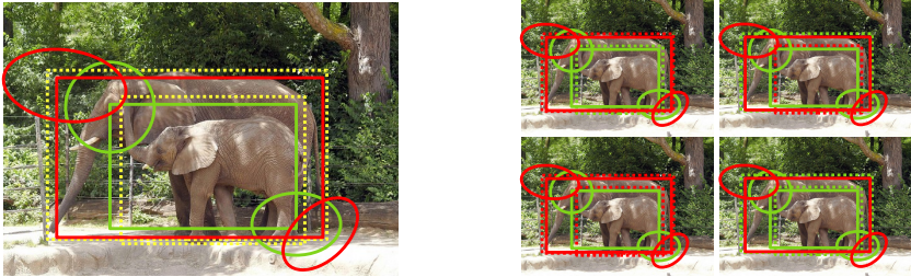
(a) Set \mathbb{Y} (yellow) with two ground truth objects and a multi-Bernoulli with two Bernoullis \mathbb{X}_1 and \mathbb{X}_2 with densities f_{B_1}(\cdot) and f_{B_2}(\cdot) . Ellipses represent uncertainties in bounding box location and shape. The large spatial uncertainties in f_{B_1}(\cdot) make it a decent description of both true objects. (b) Visualization of the four potential assignments, ordered in decreasing likelihood. In the bottom row, both ground truth objects have been assigned to \mathbb{X}_1 and \mathbb{X}_2 respectively. As f_{B_1}(\mathbb{Y})=f_{B_2}(\mathbb{Y})=0 for sets with cardinality larger than one, both these assignments have a likelihood of zero.
