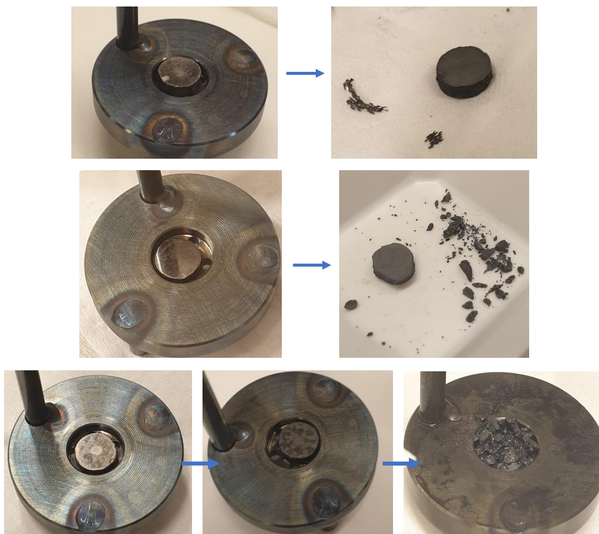
Figure 6.28. Photographs of (U80Cr20)N-3 (top), U80Cr20N-13 (middle), and U80Cr20N-23 (bottom) Cr-doped UN pellets from Batch A and B before and after exposure to water at 300 °C. The U80Cr20N-23 pellet was exposed for 3 extra hours, after which crumbling occurred.
