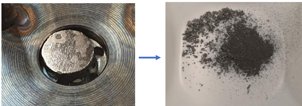
Figure 6.10. Picture of pellet UN-6 before and after water interaction. The powder was filtered from the remaining liquid and left to dry in a glovebox with <1 ppm O_2 .
