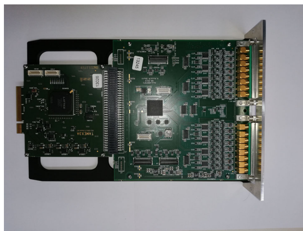
Fig. 7 New multi-channel electronic card FQT-TAMEX3. The card consists of two boards which are plugged together via a multi-pin connector. The board on the right is the front-end-electronics FQT and on the left one can see the FPGA-TDC TameX
