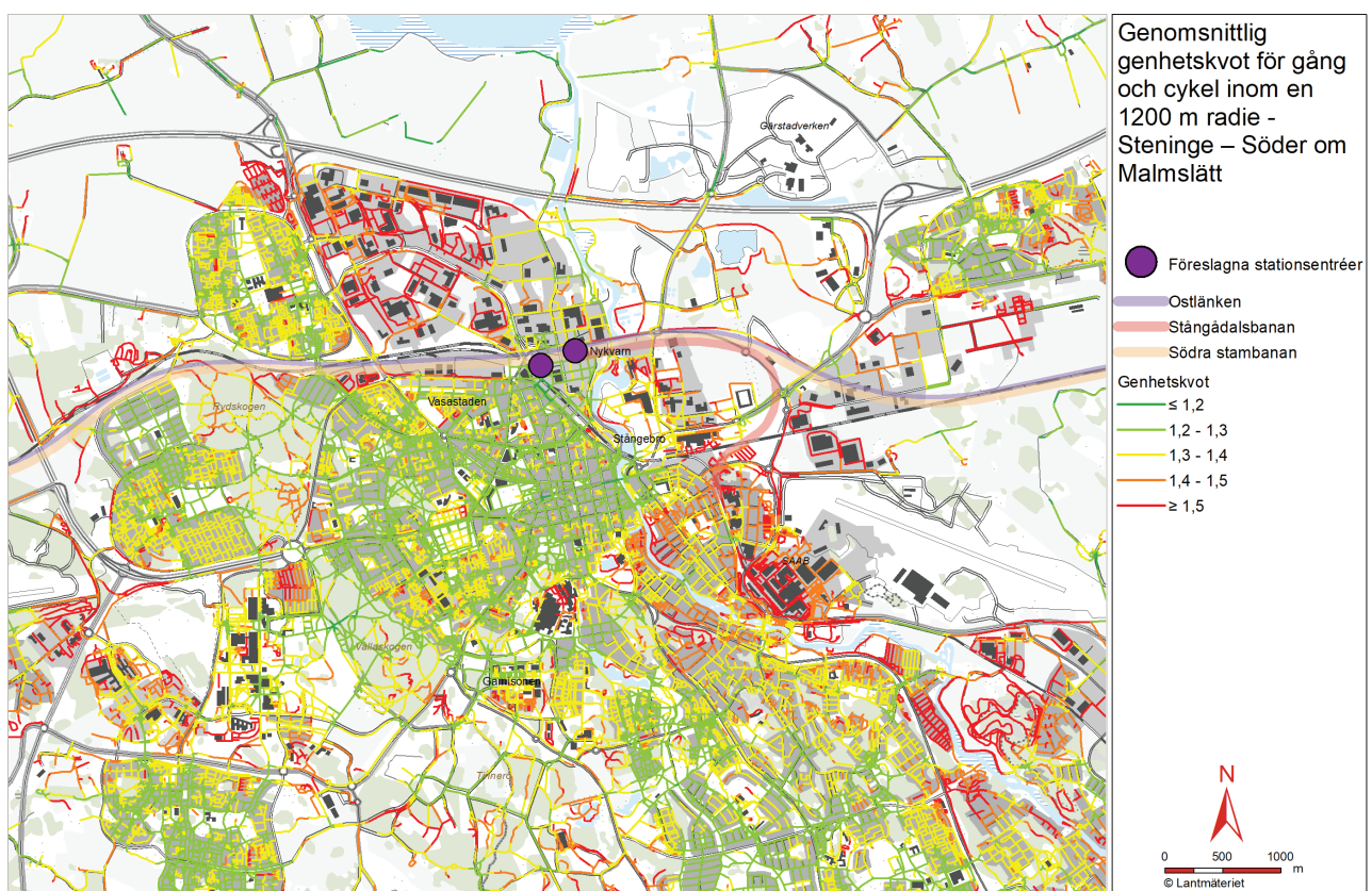
Figure 4 Example of the results of one of the BEA: Analysis of the Steninge corridor for the average detour factor for cycle and pedestrian trips within a radius of 1 200 m from each street segment. Range detour factors between \leq 1,2 and \geq 1,5 .
