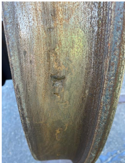
Figure 5: Wheel with isolated RCF defects
