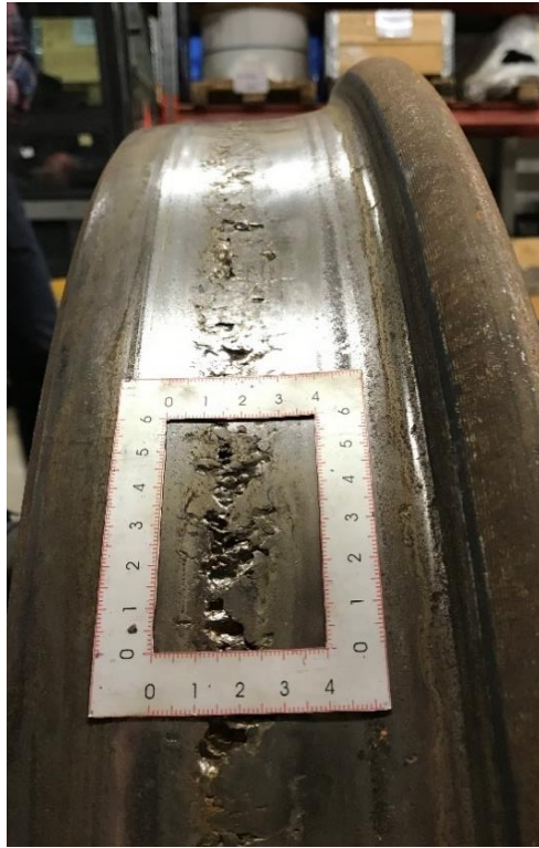
Figure 4: Wheel with severe RCF damage
