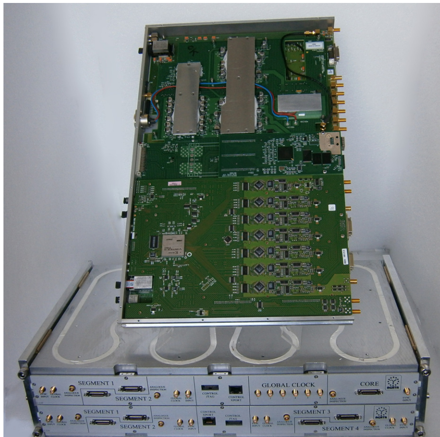
Fig. 25. (Colour online) Photograph of the AGATA digitiser.
