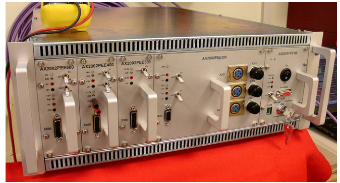
Fig. 19. (Colour online) The axis low-voltage power-supply unit generating \pm 6 V and \pm 12 V to power the 111 preamplifiers of the ATC detector, +48 V and +5 V for three digitisers, +6.5 V for three HV Modules and +24 V for the PROFIBUS-DP network.
