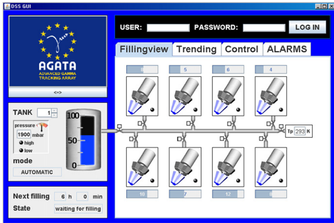
Fig. 22. The graphical user interface of the AGATA detector-support system showing the autofill page. The autofill manages detectors in groups of eight units. On the left hand side of the figure, the level of liquid in the main supply tank is shown as well as its internal pressure and the time remaining to the next programmed fill. On the right hand side, the colour of the detector endcap gives an indication of the detector temperature (blue for cold, orange for warming up, red for warm). Trending (real-time plot of any variable parameter), Control (parameter setting) and Alarms (alarm status) pages are also accessible from this GUI. (For interpretation of the references to colour in this figure legend, the reader is referred to the web version of this article.)
