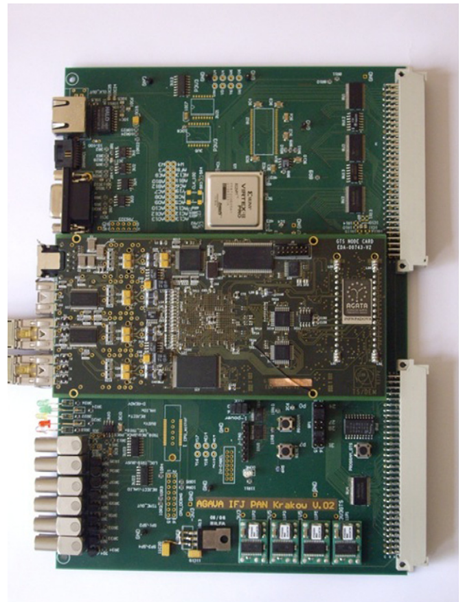
Fig. 33. (Colour online) Photograph of the AGAVA module with the GTS mezzanine card.
