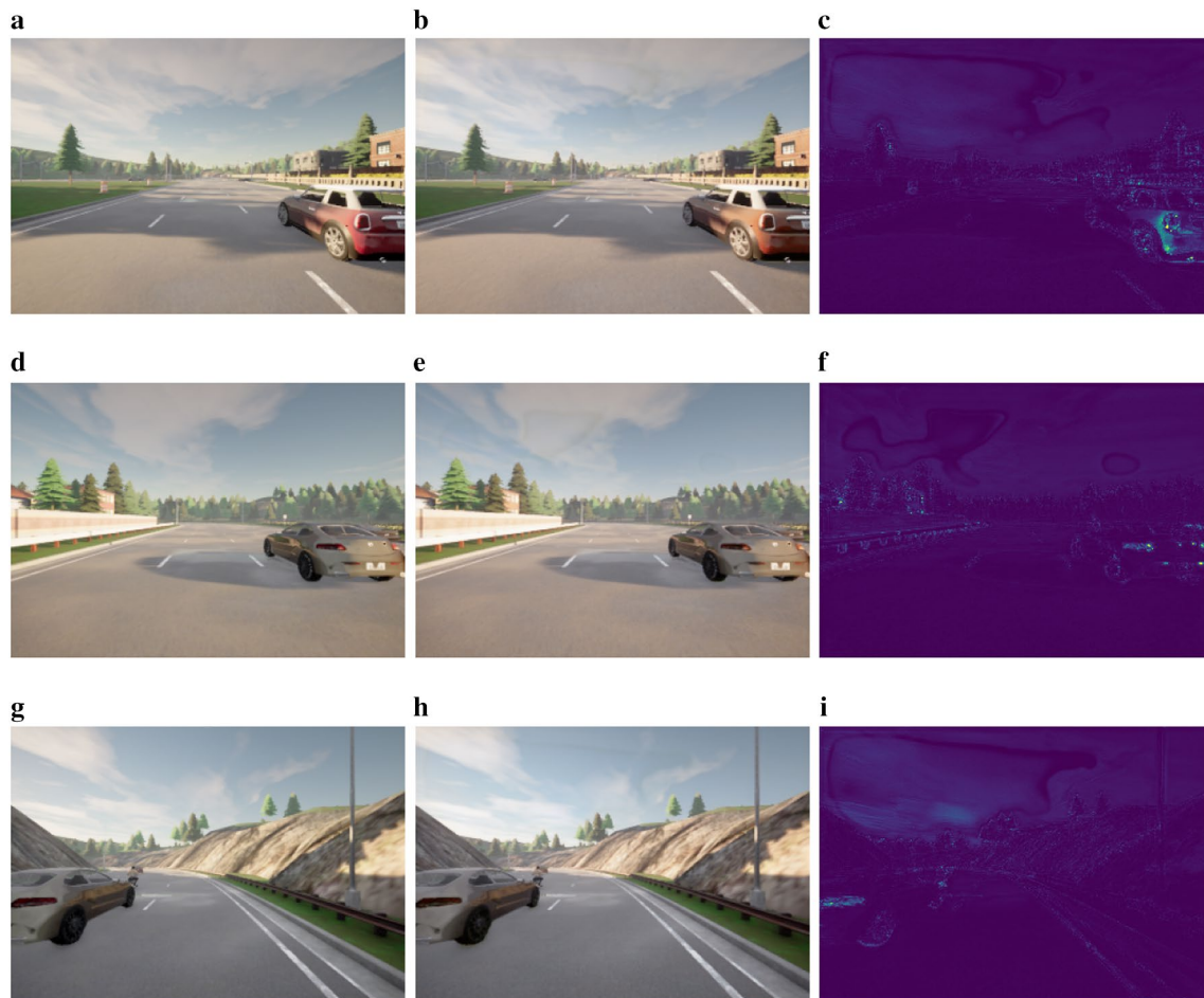
Fig. 12 Autoencoder visual example results for CARLA dataset: a input image for the anomalous driving scenario (red car), b reconstructed image for the anomalous driving scenario (red car), c reconstruction error image for the anomalous driving scenario (red car), d input image for the anomalous driving scenario (grey car), e reconstructed image for the anomalous driving scenario (grey car),
