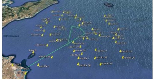
Fig. 2. Position of: the three coastal base stations ( Base # ); the additional receivers ( Add Rx # ). The simulated trajectory of the target vessel leaving the Tunisian coast and heading toward Pantelleria island is represented by a cyan line.
