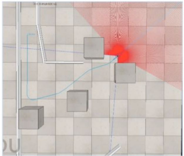
Fig. 20. Simulating obstacle avoidance behaviour robot with Laser-Landmarks sensors and FKF algorithm in V-rep software
