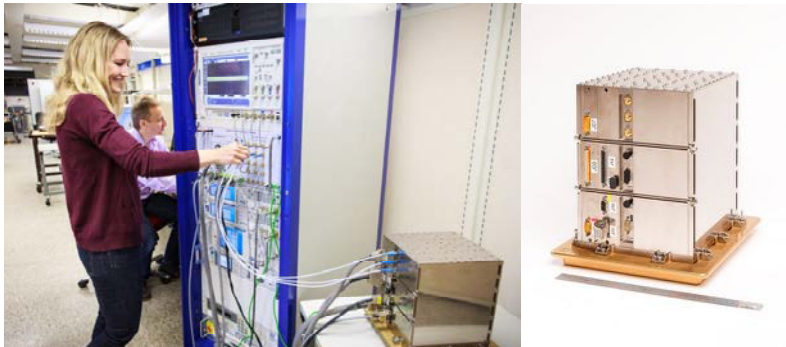
Figure 1: Studies being performed on Galileo Self-Compensating Device (SCD) engineering model that will improve the quality of the transmitted navigation signals by allowing compensation of on-board signal chain imperfections.
