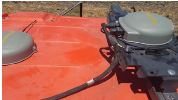
Fig 8: Topcon AGI-4 receivers used for the test (left: receiver fed by EDAS DGPS, right: receiver fed by Topcon's HiperV RTK base).
