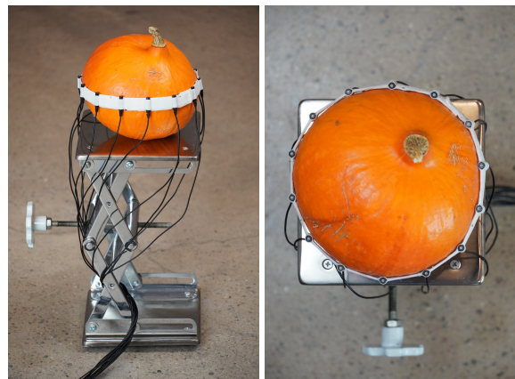
Fig. 2: Side view (left) and top view (right) of our very first prototype of an equatorial XMA based on a pumpkin. The array comprises 14 omnidirectional microphones and provides 6th ambisonic order.
